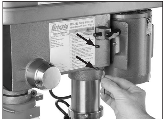
Figure 13. Securing headstock to column.
